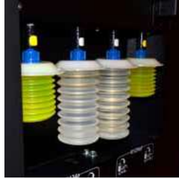
4 separate lines for oil and dye with hermetic containers
