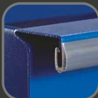
5 Double Hemmed Edges Drawer edges are hemmed to double thickness for extra stiffness.
